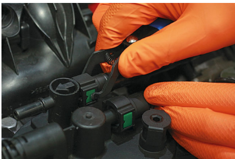
Scarab Quick Connector Disconnect Tool | 7826
